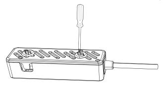
b. Use a brush to clean the heater with the cover open.
